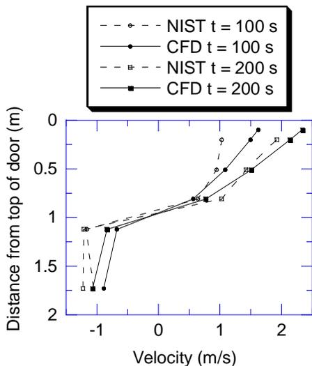
Fig. 6 Velocity profile doorway centreline at  $t = 100$  s and  $t = 200$  s.
