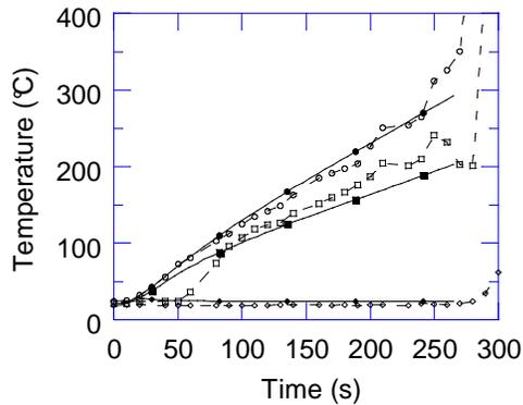
Fig. 5 Temperature stratification in doorway centreline as a function of time.
