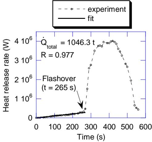
Fig. 2 Heat release rate as a function of time.
