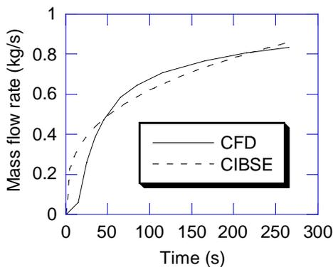
Fig. 7 Mass flow out of room as a function of time.
