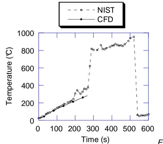
Fig. 3 Temperature in the centre of the room, 0.1 m below ceiling, as a function of time.
