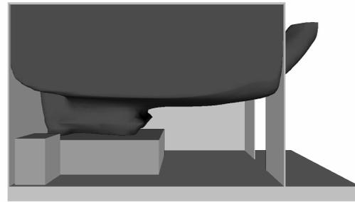
Fig. 8 Iso-surfaces of 15,000 ppm carbon dioxide at  $t = 150$  s (video available).
