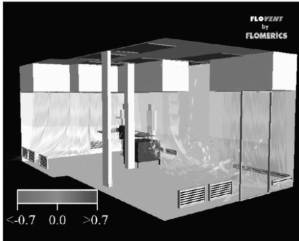
Also, one solution to the reducing upward flow in the LAF is to provide local exhaust around the corner of the room below the LAF, figure 9. This reduces the quantity of air moving off across the floor towards the fill line thus reducing the upward flow there.
