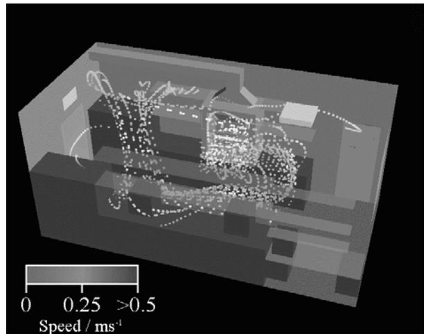
**Figure 4. Disturbed flow in front of hood**
