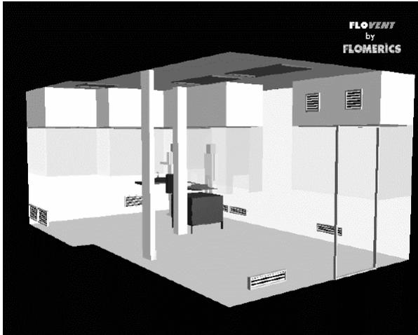
**Figure 7. Geometric model of vial filling room**
