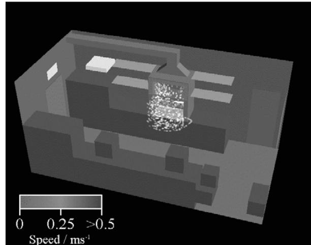
**Figure 6. Flow re-entrained in front of hood**
